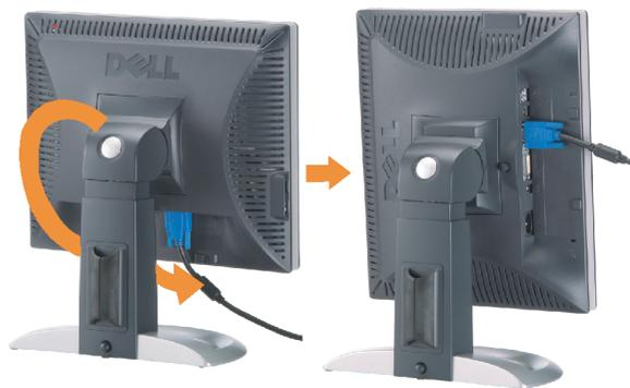
**2 Rotate the monitor to connect the cables.**
