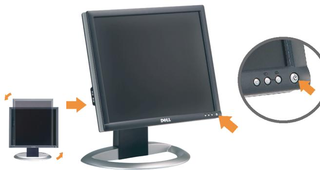
**6 Rotate the monitor back and turn on the monitor.**
